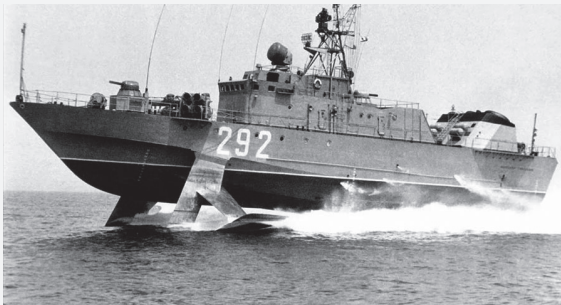
Soviet Crimea's main products. Small anti-submarine ships (corvettes) of the project 1145.1, codename Sokol, NATO class Mukha. A series of small anti-submarine ships built at the Feodosia Morye shipyard since 1987. A unique design of a warship on submarine wings. Photos from the Blackseanews archive
