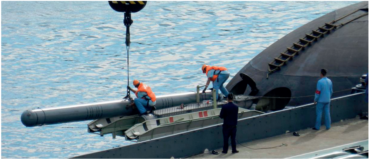
Loading of the Caliber cruise missiles into the torpedo-launching device of the new project 636 submarine of the RF BSF. Sevastopol, September 2, 2017. Russian Black Sea Fleet, Sevastopol, September 2, 2017, Yuzhnaya Bay, photos from social media
