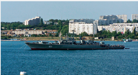
Soviet Crimea's main products. Missile frigates of the project 1135, multipurpose ocean ships, codename Burevestnik, NATO class Krivak. Kerch Plant Zaliv has built 15 of them in 1971-1991. Photo by A. Brichevsky, www.kchf.ru
